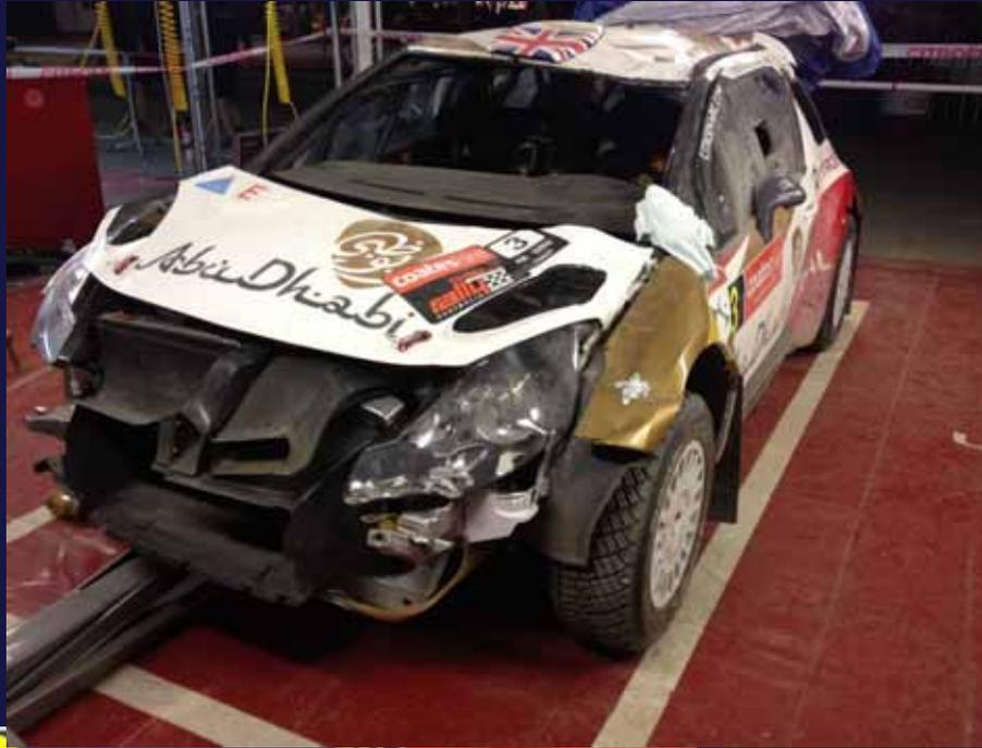
Check if rollcage is damaged before the team starts to repair the car !!!
