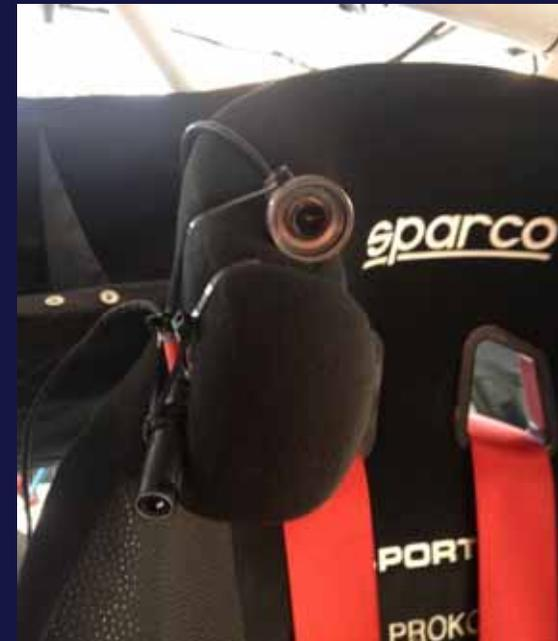
Inboard camera must be fitted properly / safely
