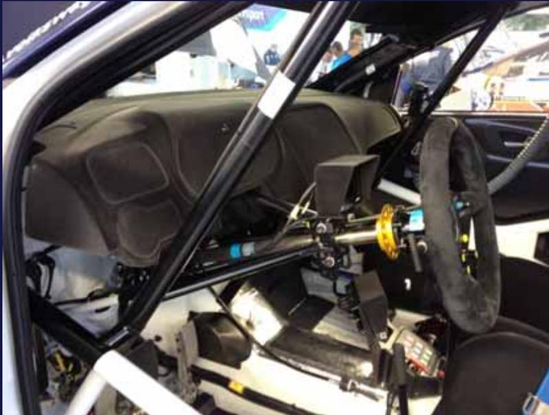
**R5:** The quick release mechanism is compulsory and must consist of a flange concentric to the steering wheel axis, coloured yellow through anodisation or any other durable yellow coating, and installed on the steering column behind the steering wheel.
