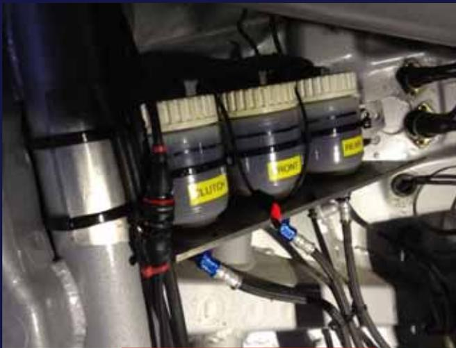
If brake fluid / clutch fluid tanks are fitted inside the cockpit, they must be protected by a leakproof and flameproof cover.
